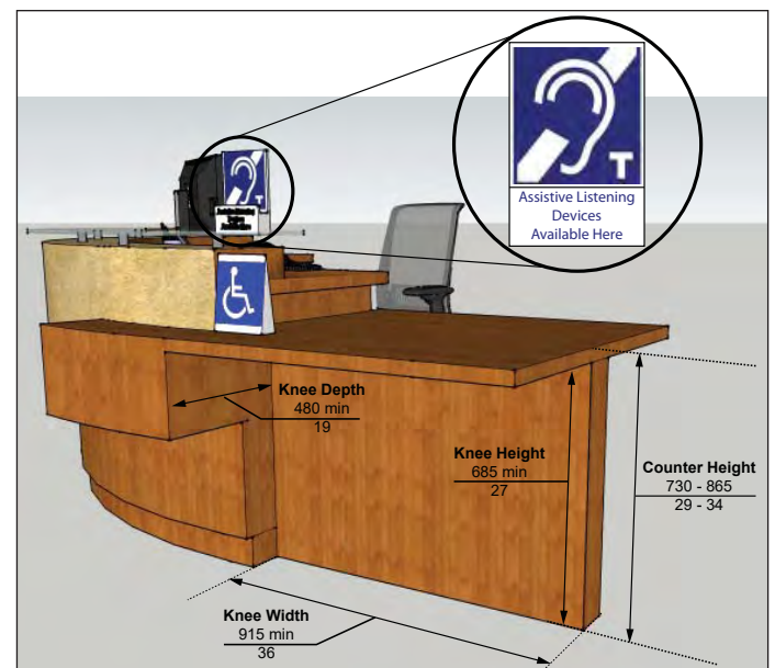
Figure 93: Dimensions of Accessible Service Counter
