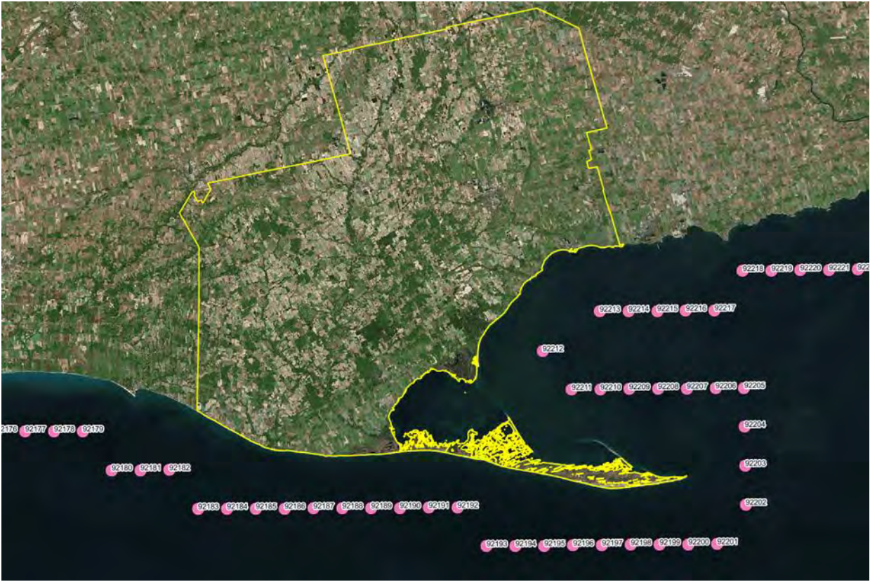
Figure 3.3: Wave hindcast output points from the US Army Corps of Engineers Wave Information Study
